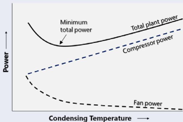
To implement variable cooling water temperatures at Fonterra, both a dry bulb temperature sensor and a relative humidity sensor were installed. This enabled a wet bulb temperature to be calculated, which is used to calculate the desired condensing temperature set-point. To reach this condensing temperature, the plant Programmable Logic Controller (PLC) varies the speed of the cooling tower fans.
